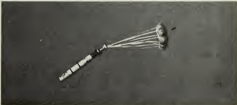
PARACHUTE TORPEDO—Mark 44 torpedo is a new lightweight ASW weapon that seeks out target. It can be dropped by plane or fired from shipboard.
